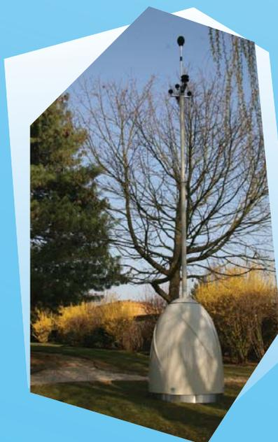
**The Sonopode®** is a specific equipment that has been developed by Bruitparif to make the installation of a noise measurement station easier, particularly in the case of air noise nuisances where the expert stations used require a solidly anchored mast. It requires no connection thanks to:
